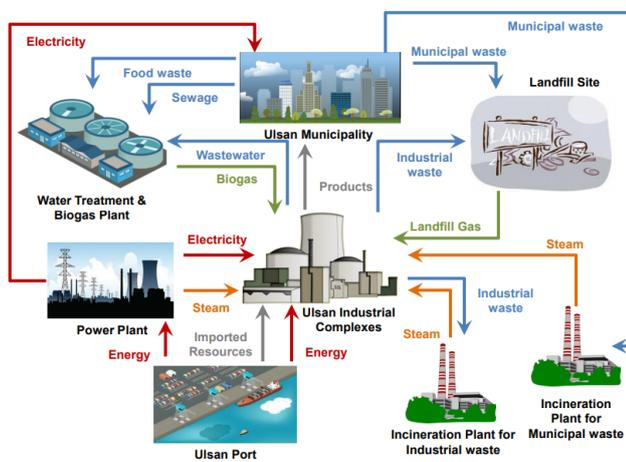
Fig. 3. Simple diagram of the resource exchanges within the city of Ulsan and its municipality [52].
