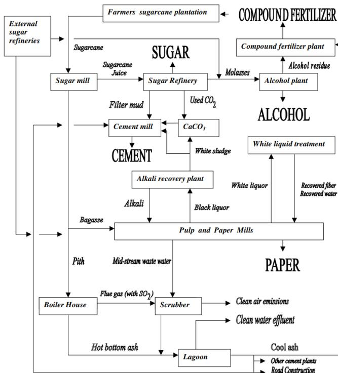
Fig. 1. Diagram of resource exchanges in Guitang group using only the organisation’s wastes and by-products [43].
