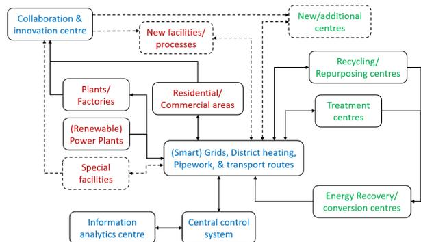
Fig. 5. The detailed subsystems of the conceptual framework and the relationships between them. The solid lines denote established subsystems and relationships whereas the dotted lined denote the potential for that subsystem, or relationship.
