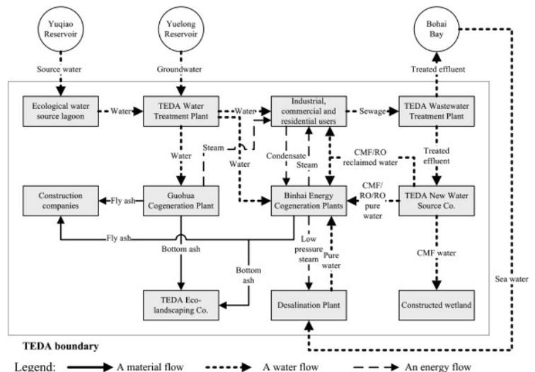
Legend: — A material flow    - - - - - A water flow    ······ An energy flow
