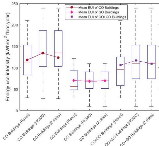
Fig. 5. EUI of the buildings in Hanoi and HCMC.
